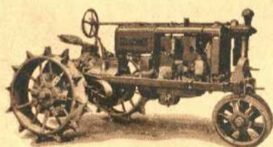
The big 3-plow Farmall 30. There is also the original 2-plow Farmall.
