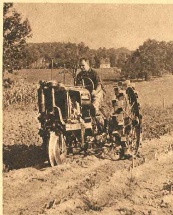
The New Farmall 12 provides all-purpose Farmall power in a size to fit small farms. Has the features and advantages of the original Farmall tractor, scaled down in size, weight, power, and price. Pulls a 16-in. or two 10-in. plow bottoms. Has capacity of 25 to 33 acres a day in planting and cultivating corn, cotton, etc. Uses your own equipment and special Farmall equipment.
